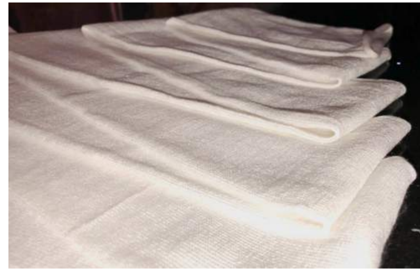
Nullarbor fabric made from microbial cellulose
